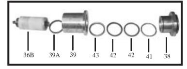
5. Take seal case (38) out of seal sleeve (39). Examine plunger parts (36A-36D), seals (42,39A) and O-rings. When replacing plunger pipe (36B), tighten tension screws (36C) to 30 ft. lbs.
